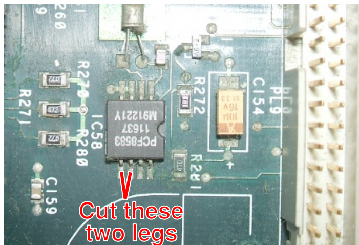
The clock chip on the A5000 motherboard, just above the battery
