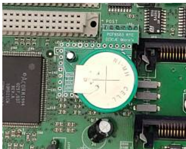
Location of the RTC Module on the motherboard, to the right of the Processor sockets.
