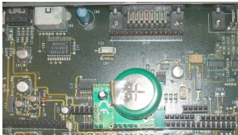
Fit the clock module here
