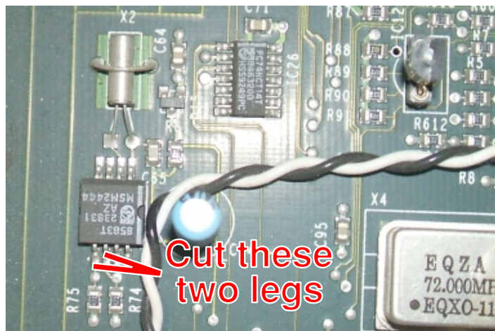
The clock chip on the A30x0 motherboard, just in front of the keyboard connector
